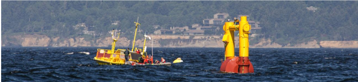
Figure 3. Deployment of the umbilical cable connecting the WET-NZ device under test to the Ocean Sentinel at NNMREC's open-ocean test site north of Newport, OR.
