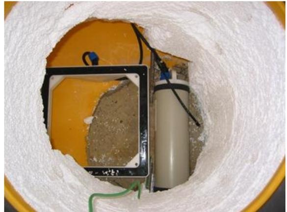
FIGURE 4: The topside WFS modem was mounted internal to the buoy hull, below the battery pack near the waterline deemed to be a safe location from fouling/corrosion.
